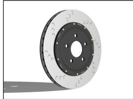
The STāSIS brake assembly replaces the 330 mm 1 piece cast iron rotor with a 2 piece 330mm rotor consisting of an aluminum hat and light weight rotor. Weighing in at just 13.3 pounds, the new assembly removes approximately 4 pounds of rotating weight at each corner. Compared to the OEM rotor, the STāSIS rotor features directional slotting to whisk away pad material and water.
